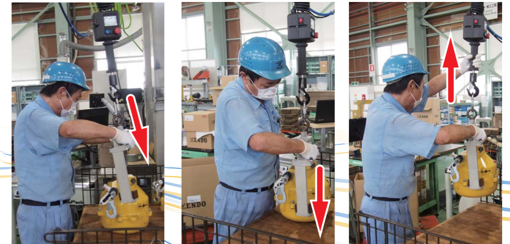
Manual operation sets the jig smoothly
