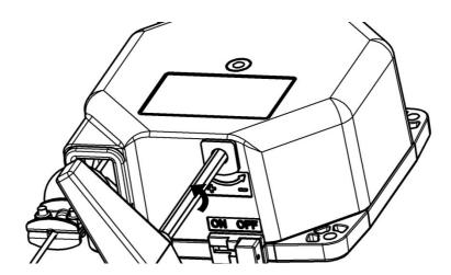
5 Remove the bolts and remove the cover.
