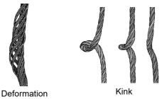
Note: Kink is the state in which the wire rope is partially deformed due to torsion or looseness.
