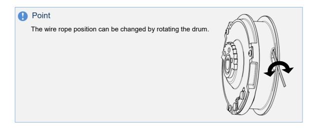
6 Assemble drum, drum cover and wire rope.
