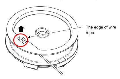
Remove the plates from the edge of wire rope.
