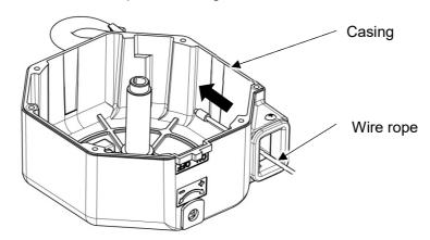
2 Insert the new wire rope into the drum.
