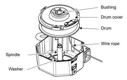
7 Turn the drum over and lift up the edge of wire rope using a flat head screwdriver.
