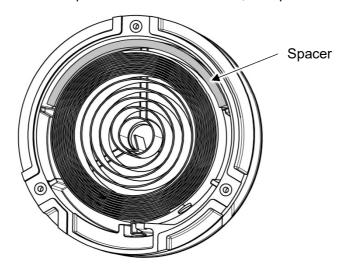
3 Put grease to the top surface of the spring.
