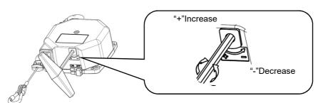
If you would like to limit the winding length, change the stopper position, but do not set below the factory set position.
