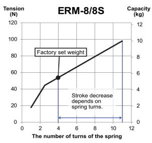
1 turn of the spring ≒350mm wire rope extraction 1 turn of the spring=14 turns of worm
