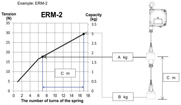
1 turn of the spring ≒350mm wire rope extraction
