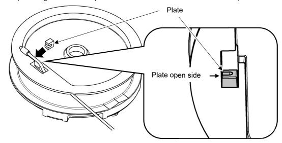
4 Pull the wire rope and fix the wire rope and plate into the notch of drum.
