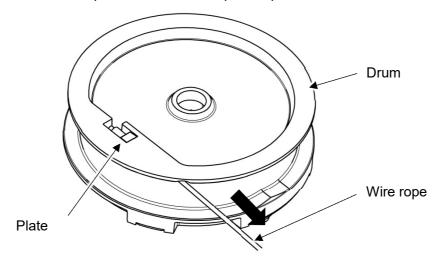
5 Make sure the wire rope is parallel to the side of the drum.
